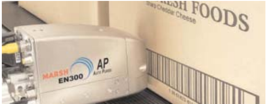
Using a high-resolution, large character ink jet printer for graphics, numerical codes and barcodes companies can eliminate the need for pre-printed boxes.
